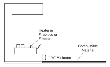
Figure 11 - Minimum Clearance above Combustible Flooring
